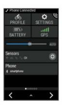
The settings widget appears. A flashing icon means the device is searching. You can select any icon to change the settings.
