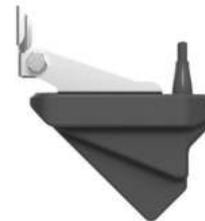
**NOTE:** To use the compass, you must mount the transducer on the transom or the trolling motor shaft. The compass may not work when you mount the transducer on the motor.
