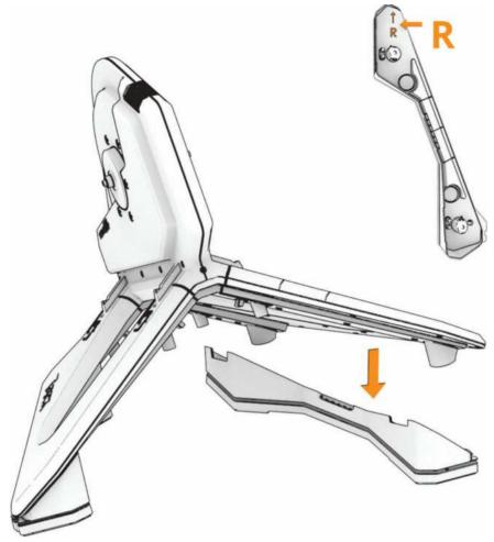
5 Check the alignment of the plates on both sides.
