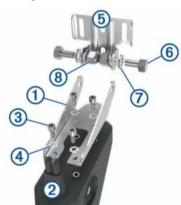
Attach the transducer mount bracket to the transom mount bracket (5) using the bolts (6), flat washers (7), and lock nuts (8).
